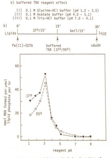
Conclusion: pH 3.5 is optimal for formation of TBA-reactive products from lipid hydroperoxides.
