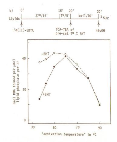
Conclusion: Gradual warming of the incubation mixture from room temperature to boiling favours the breakdown of hydroperoxides to generate TBA-reactive substances. Hot TBA (95°) inhibits breakdown of hydroperoxides to TBA-reactive products.
