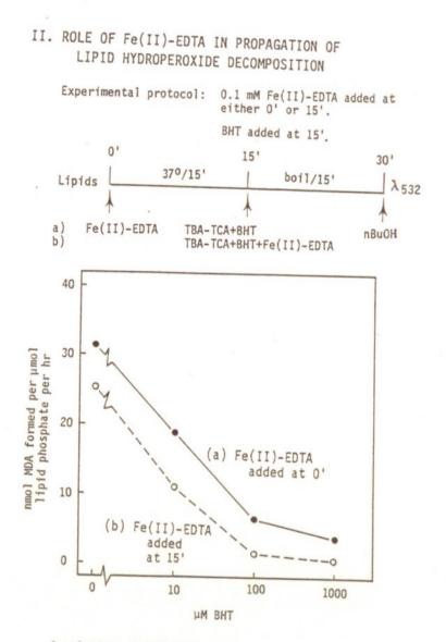
Conclusion: Fe(II)-EDTA catalyses thermolytic breakdown of lipid hydroperoxides to form TBA-reactive products.
